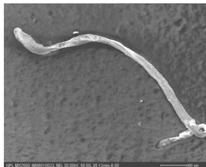
Particle IMO8010023 (beta rich; high Fe component)
